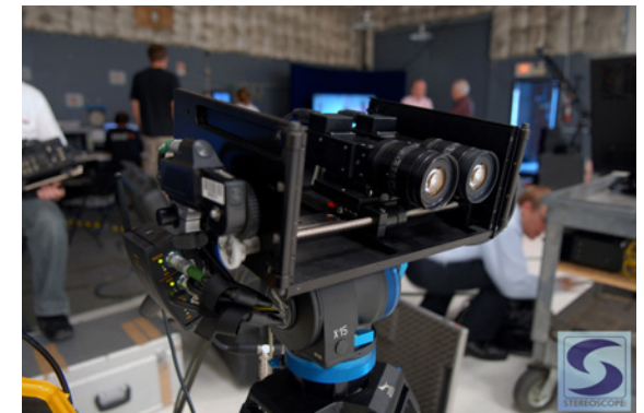
A small side by side rig designed to support the small Cunima cameras. The small camera bodies and lenses allow this rig to have a smaller minimum interaxial distance. Image courtesy of Stereoscope.
