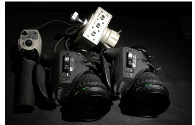
Most 3D lens systems are designed to operate both lenses with a single controller.
