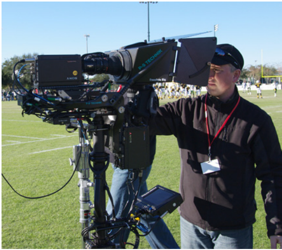
A mobile beam splitter rig designed to be used with a Steadicam. Image courtesy of ZGC.
