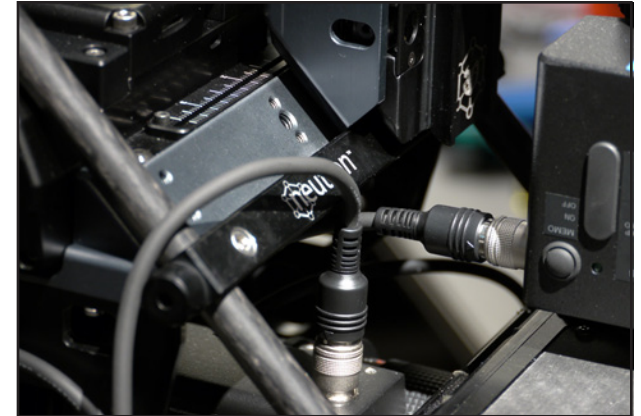
Improperly fitted cables on a rig
