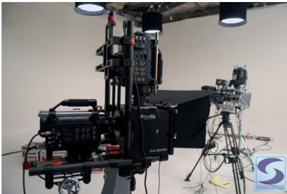
A studio beam splitter rig designed for tripod or dolly use. Image courtesy of Stereoscope.
